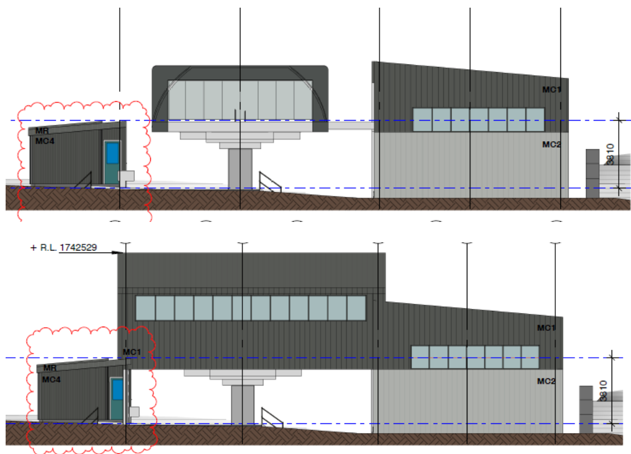
Figure 5 | Elevation view of bottom station and carrier shed, with proposed Stage 1 (top without enclosure) and Stage 2 works illustrated (Source: Applicant's documentation)
